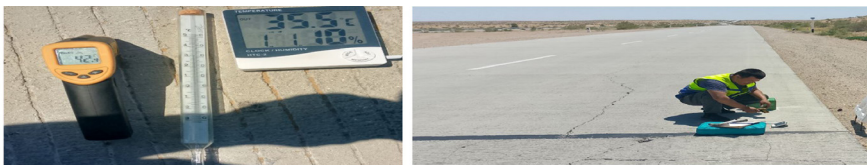
Figure 1. Showing air temperature, surface temperature, and bottom temperature of the plate
